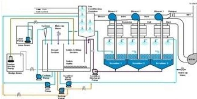
*Schematic of the ENVI-Clean™ Emission's System as installed for Biomass applications*
