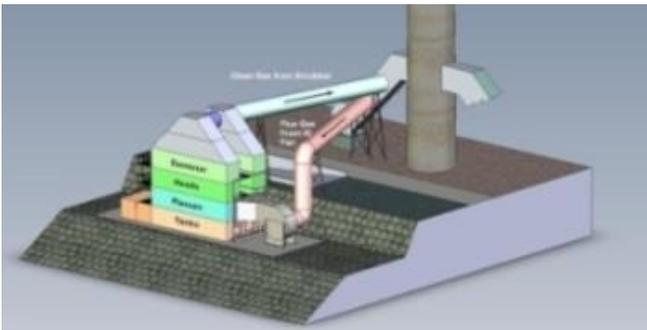
The ENVI-CES™ technology forces 100% of the polluted exhaust flue gas into the neutralizing fluid to produce a highly turbulent interaction between the target pollutants and the fluid. The aggressive mixing produces small bubbles which create a very high surface contact area between the exhaust gas and fluid to enhance the transfer of particulate and targeted gaseous and hazardous pollutants from the exhaust to the fluid.
